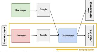
Fig. 5. Flow of the entire process with respect to generator loss
